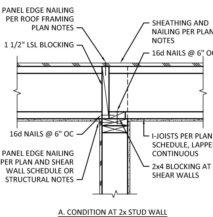
**1** ROOF FRAMING DETAIL (INTERIOR BEARING AT SHEAR WALL)
