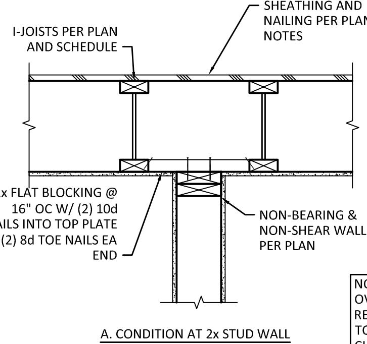
**4** ROOF FRAMING DETAIL (INTERIOR NON-BEARING AT NON-SHEAR WALL)
