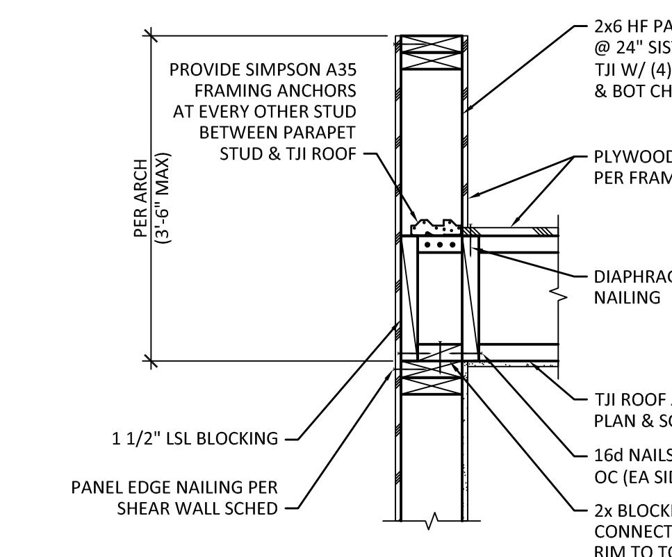
**5** FLAT ROOF SECTION W/ PARAPET
