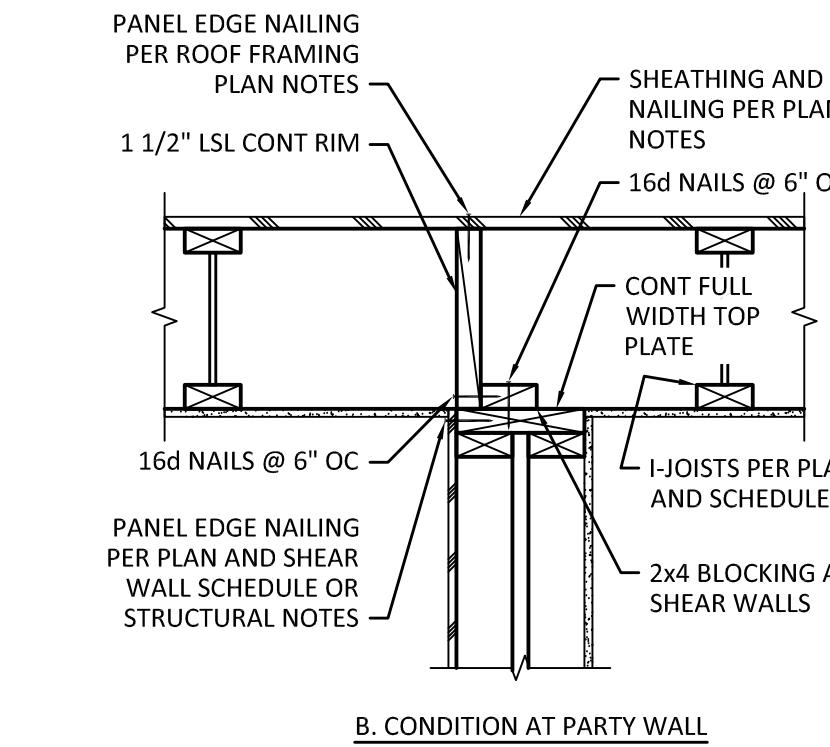
**2** ROOF FRAMING DETAIL (INTERIOR NON-BEARING AT SHEAR WALL)
